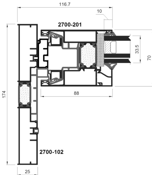
Fig. 8 Cross section test specimen -08\*
