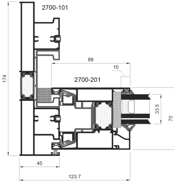
Fig. 1 Cross section test specimen -01\*
