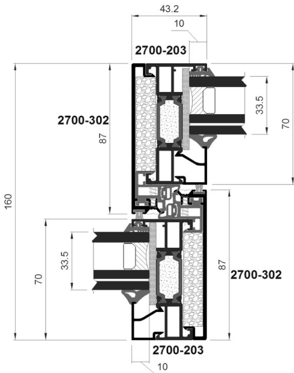
Fig. 6 Cross section test specimen -06\*
