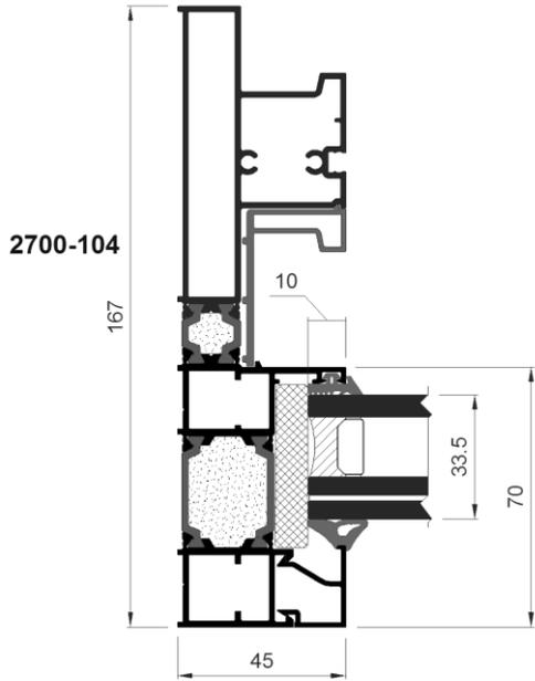
Fig. 5 Cross section test specimen -05\*
