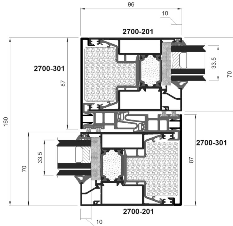
Fig. 3 Cross section test specimen -03\*
