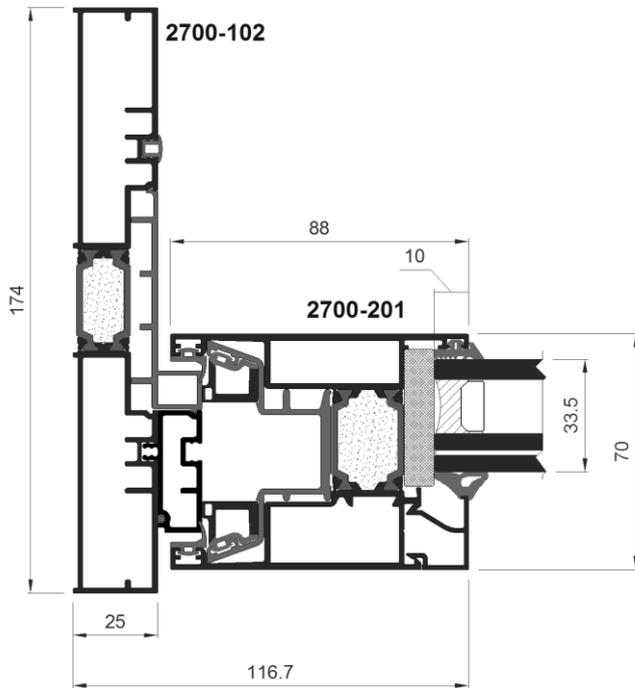
Fig. 7 Cross section test specimen -07\*
