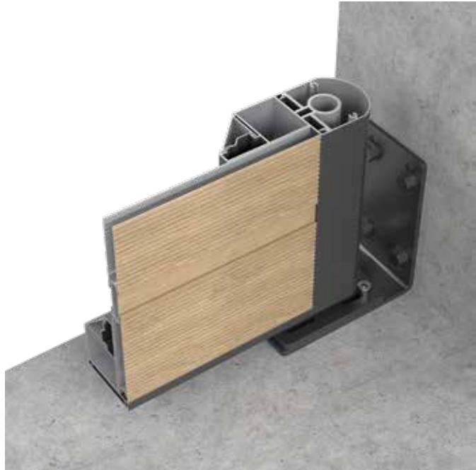
Detailed views of the sash and grooved profiles, along with the pivot axis profile with INOX 316 PIN able to hold 250 kg each. Maximum single door sash is close to 4m<sup>2</sup> withstanding a maximum wind load of 2KPa.
